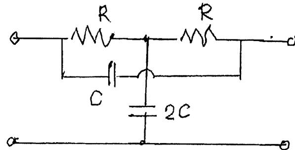
2. Two of the short-circuit admittances of the circuit shown are  $y_{11} = y_{22} = (7s^2 + 1)/(16s^3 + 4s)$ . Find all element values.
